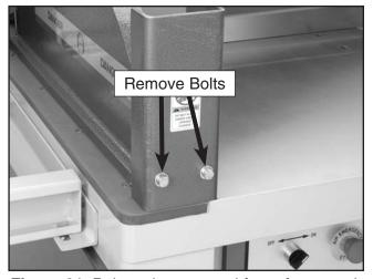
Figure 21. Bolts to be removed for safety guard.
